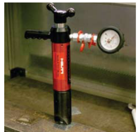
Pullout test of an ENP fastening with a Mark V tester and ENP adapter.
