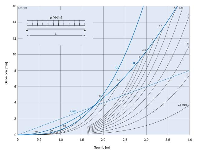
M ... permitted bending moment Q ... permitted shear force p ... actual load (service load)
