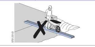
Do not use as holding girders (heavy point load in conjunction with wide span).
