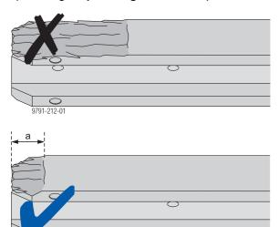
Damage to the plastic cap has no effect on loadbearing capacity, but beams evincing damage of this kind do not necessarily meet the quality criteria for Doka rental formwork.
