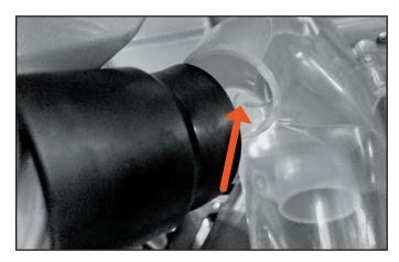
Slip upper vacuum hose onto dust guard inlet.
