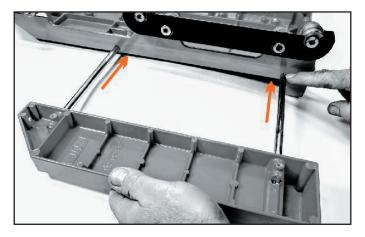
With a Phillips screwdriver, install screws in each end of extension shaft to secure.
