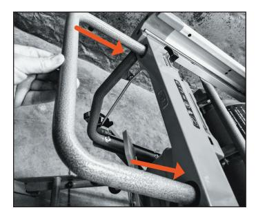
Insert lock screws into handle and tighten.
