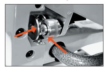
Put the remove table lock lever in the up position. The remove table lock lever should remain in the up position for normal operation. The remove table lock lever should only be put in the down position for table removal and maintenance.
