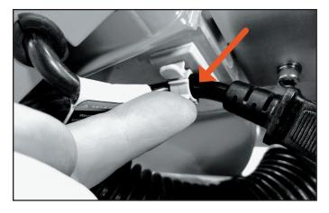
Plug the vacuum power cable into the vacuum power supply receptacle.
