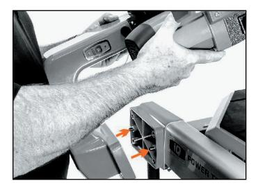
Install the (4) Allen screws. Tighten all 4 screws finger tight.
